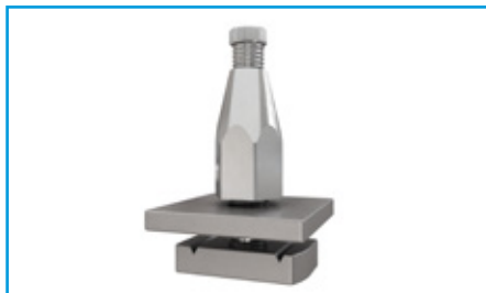
Trapeze Plus No. 3 Combine Trapeze Plus as an accessory with any Trapeze kit for multi-tiered installations. Load rating of 90 kg with a 3:1 safety factor. Product code: GRIPPLE3MM-TPZ-METAL
