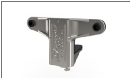
Duct Trapeze Ideal for use with rectangular ductwork. Combine Duct Trapeze as an accessory with any Trapeze kit for multi-tiered installations. Maximum load rating of 45 kg with a 5:1 safety factor. Product code: DT2-ACC-PAD
