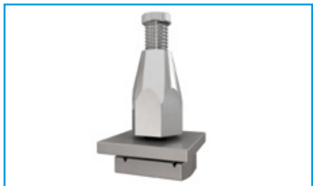
Trapeze Plus No. 4 Combine Trapeze Plus as an accessory with any Trapeze kit for multi-tiered installations. Load rating of 225 kg with a 3:1 safety factor. Product code: GRIPPLE4MM-TPZ-METAL
