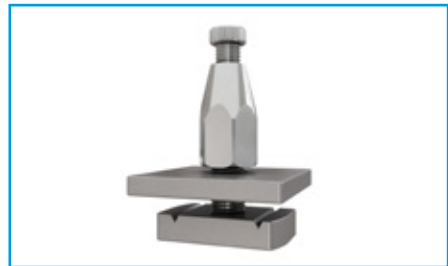
Trapeze Plus No. 2 Combine Trapeze Plus as an accessory with any Trapeze kit for multi-tiered installations. Load rating of 45 kg with a 3:1 safety factor. Product code: GRIPPLE2MM-TPZ-METAL
