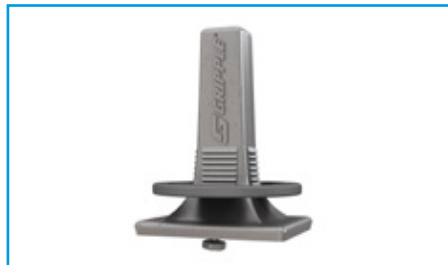
Trapeze No. 2 Combine Trapeze as an accessory with any Trapeze kit for multi-tiered installations. Load rating of 45 kg with a 3:1 safety factor. Product code: TRAPEZE-NO2
