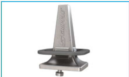
Trapeze No. 3 Combine Trapeze as an accessory with any Trapeze kit for multi-tiered installations. Load rating of 90 kg with a 3:1 safety factor. Product code: TRAPEZE-NO3
