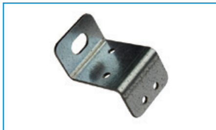
Trapeze Bracket Combine with Trapeze No.2 and No.3 for easy attachment to rectangular ductwork. Maximum load rating of 45 kg (No.2), 90 kg (No.3) with a 5:1 safety factor.
