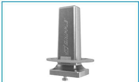
Trapeze No. 4 Combine Trapeze as an accessory with any Trapeze kit for multi-tiered installations. Load rating of 225 kg with a 3:1 safety factor. Product code: TRAPEZE-NO4
